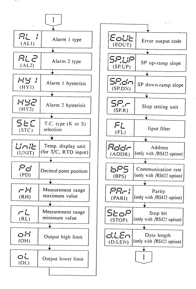
CAUTION: The parameters shown below are automatically initialized when the value of STC and/or UNIT is changed.
