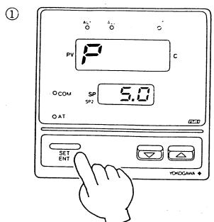
From the operating parameter setting display panel, press the set key several times to come to the display in the figure at left.
