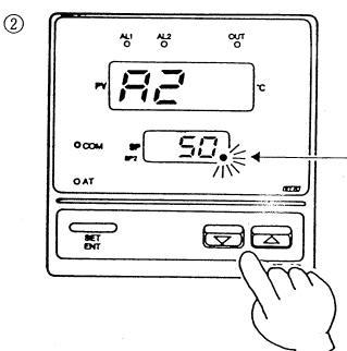
Using the and keys set the alarm 2 setting to the required value.
