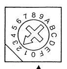
Set rotary switch **B** to the desired control output type code No. (In the example, the switch is set for continuous output PID.)
