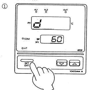
From the operating parameter setting panel, press the SET key several times to come to the display in the figure at left.
