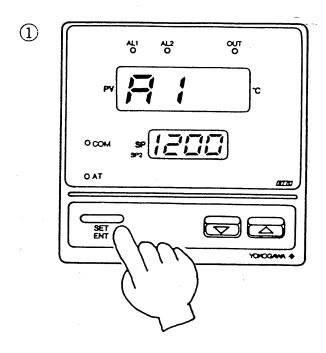
From the normal display panel (measured-value display), press the SET key for 3 seconds or more continuously. (The display should appear as at left. Verify that R: is displayed.)
