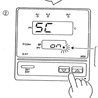
Use the and keys to display either "ON" or "OFF in the lower indicator.
