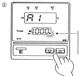
Using the and keys set the alarm 1 setting to the required value.
