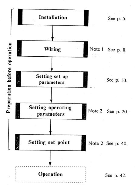
Note 1: This instrument itself has no power switch. It will begin to operate and generate a control output as soon as power is supplied to it. We recommend that the device to be controlled not be connected until immediately before operation is to begin.
