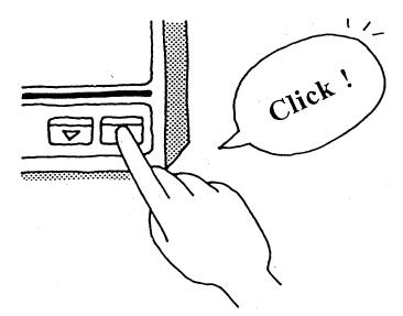
② Never use a sharp point to press the keys, as this can cause failure of the key.
