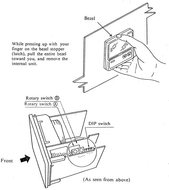
(3) When changes to the input, output, and control actions have been completed, return the internal unit to the case, and apply power.
